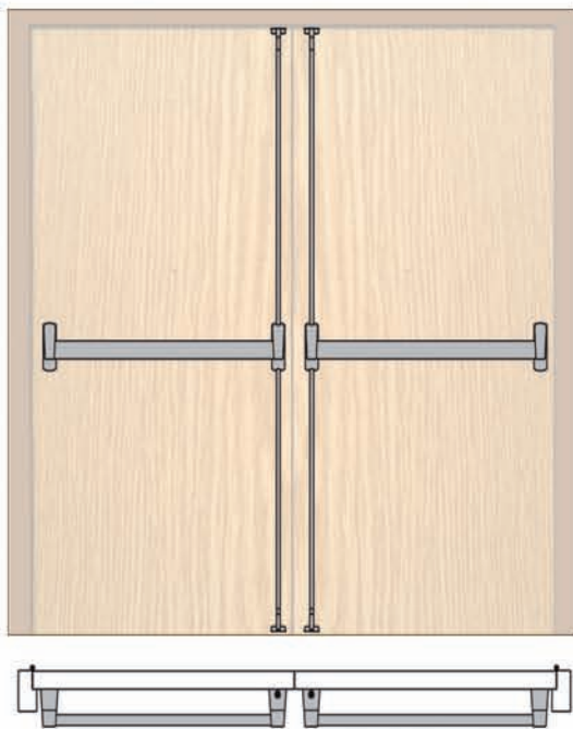
801 x 2 Non-rebated doors - for use on doors in buildings accessed by the public, where panic can be foreseen
