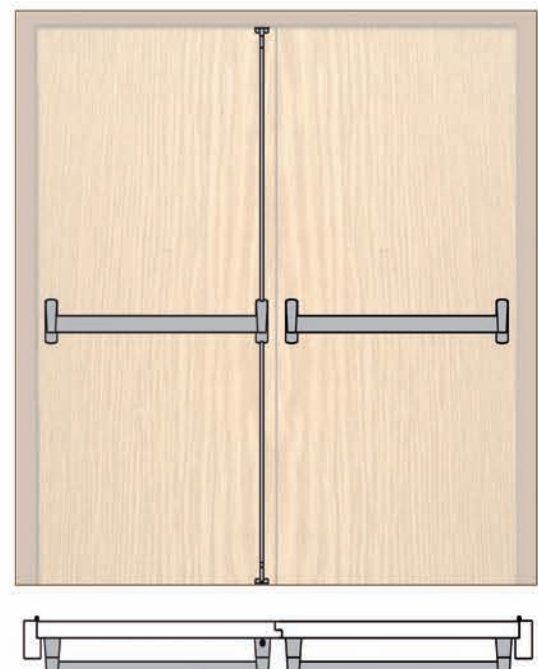
802 Rebated doors - for use on doors in buildings accessed by the public, where panic can be foreseen
